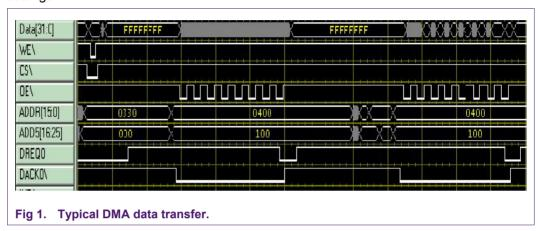
It is observed that DREQ is immediately asserted after the ISP176x DMA is enabled and the system will assert DACK in response, executing a burst according to the programmed parameters. DREQ will be deasserted on the last write or read cycle of each burst, and will be reasserted until the programmed transfer count is completed.
